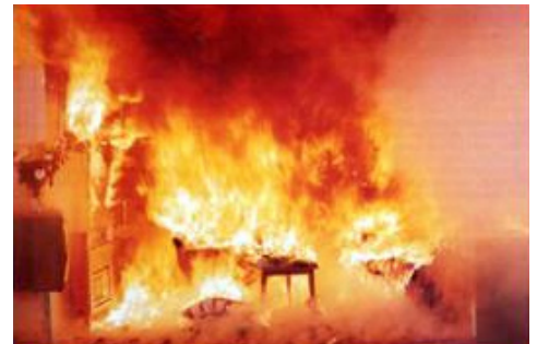
Fire in room at flashover Source: AH Buchanan
