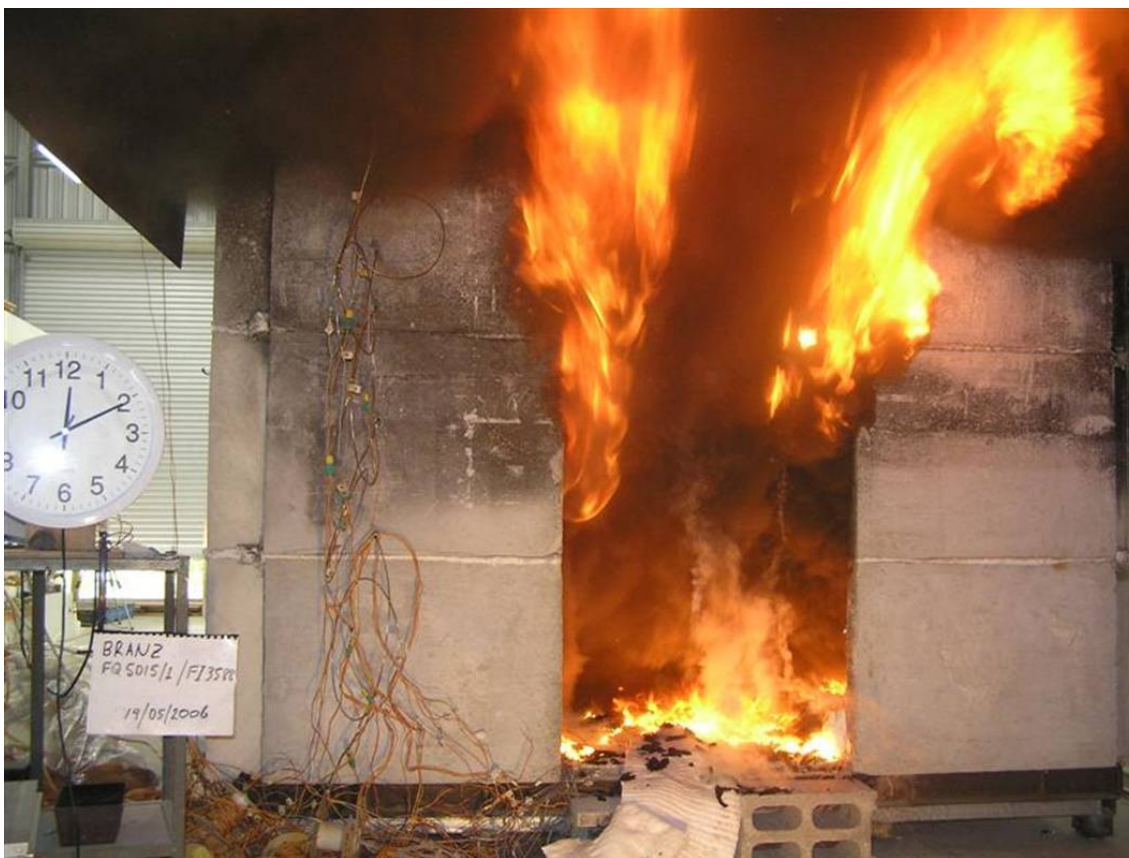
After flashover in the ISO 9705 room corner test of plywood wall and ceiling linings
